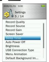
2. Use / buttons until you reach the desired time delay and press (Adjustment range: 10 Minute ~ 180 Minute or Off)
