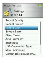
2. Use the \_\_\_\_\_ / \_\_\_\_ buttons to select your desired amount of gain and press \_\_\_\_\_ to confirm. Adjustment range: 1 ~ 7 or Off (7=highest gain, 1=lowest gain)
