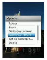
3. Use the buttons to select the effects (Normal, Slide, Chessboard, Blink, Wipe, Window Blinds, Thin Lines, Random) you want, press to confirm.
