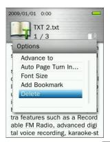
3. Use the \_\_\_\_\_ / \_\_\_\_ buttons to highlight "OK" and press \_\_\_\_\_ to delete the text file currently open, or select "Cancel" to return to the Options menu without deleting.
