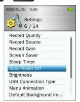
2. Use / buttons until you reach the desired time delay and press to confirm. (Adjustment range: 10 Minute ~ 180 Minute or Off)
