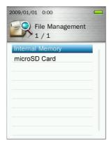
4. Use the \_\_\_\_\_ / \_\_\_\_ buttons to scroll up and down through the available folders and files in the root directory of the selected storage device.
