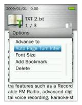
3. Use the \_\_\_\_ / \_\_\_ buttons until you reach the desired interval time of pages turning automatically and press \_\_\_\_ to confirm. (Adjustment range: 3 Sec, 6 Sec, 9 Sec, 12 Sec, 15 Sec)
