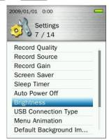
2. Use / buttons until you reach the desired level of brightness and press (Adjustment range: 1 ~ 5)
