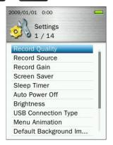
2. Use the \_\_\_\_\_ / \_\_\_\_ buttons to select Low, Medium, or High quality and press \_\_\_\_\_ to confirm.
