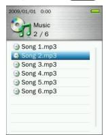
6. Use the hold / buttons to select "OK" and press to remove the song (note: this will only remove the selected song from the current playlist, and will not actually delete the file from the microSD card or internal memory).
